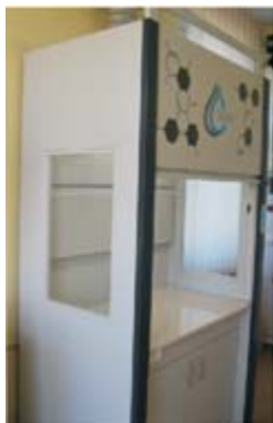
Fume hood with glazing on both sides
