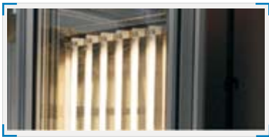
FIT D - Climatic chambers with lamps installed in the door
