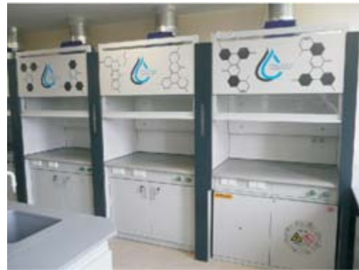
Fume hood with reduced height, to be installed in rooms with lower ceilings.
